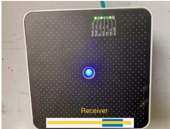
RFID Receiver to be installed on a train
